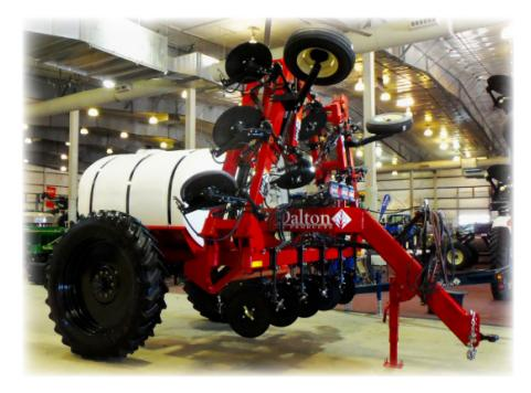
The DLQ Series Liquid Applicator is built tough for the most rugged terrain. The 4"X6" tubular main frame and the 4"X6" front mount toolbar gives you the strength and visibility you need in today's environment.
